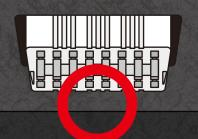
\*The connector is located on the lower right or left of the driver's seat
